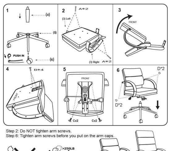
Step 2: Do NOT tighten arm screws.
